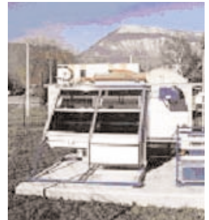
Figure 5. View of the test box for outdoor exposure and meteorological instruments at CSTB.
