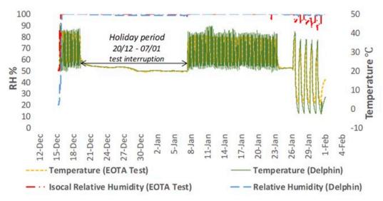
Figure 3. Comparison between Delphin results and EOTA wall test.
