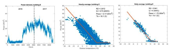
Figure 7. Building D, measured hourly values of power (left), results of hourly change-point model (middle) and daily change-point model (right).
