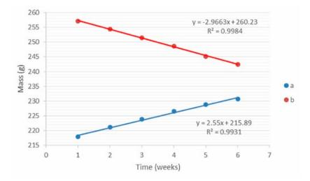
Figure 2. Examples of mass gain/loss curves for dry and wet cup tests: (a) dry cup, uncarbonated NHL5 mortar, (b) wet cup, carbonated NHL3.5.
