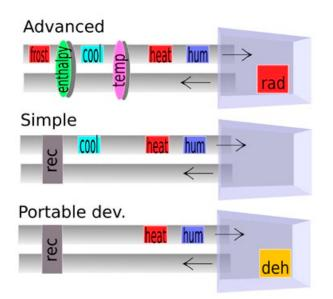
Figure 2. Three HVAC systems installed in the analysed historical buildings: frost – heating coil that preheats air; enthalpy – enthalpy wheel; cool – cooling coil; temp – thermal wheel; heat – heating coil; hum – steam electric humidifier; rad – radiator; deh – dehumidifier; rec – recirculation.
