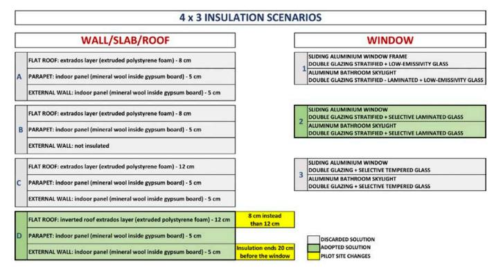
Figure 7. Different scenarios for the insulation of wall, slab, roof and windows.
