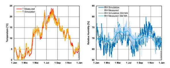
Figure 4. Measured indoor climate of the pipe organ storage vs. results from hygrothermal whole building simulation with WUFI Plus from January 2013 to January 2014. The Temperature is very well represented by the simulation and also the general level of RH even though here are some minor deviations.
