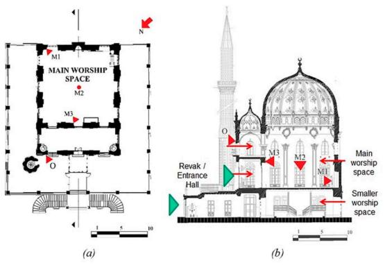
Figure 2. (a) First floor plan of the mosque and location of measurement points in horizontal plane (M1, M2, M3, O), (b) cross-section of the mosque and location of measurement points in vertical plane (M1, M2, M3, O). Source: Modified from the drawings provided by ENVAR Architecture and Engineering Inc.
