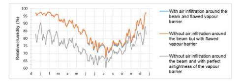
Figure 5. Impact of air infiltration around the beam end and of realistic flaws in airtightness for a configuration with cement lime plaster as external coating and cellulose wadding as insulation material. (Indicator C)
