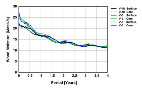
Figure 11. Course of the wood moisture of the three restoration variants calculated with WUFI<sup>®</sup>–2D for a period of 4 years after installation.
