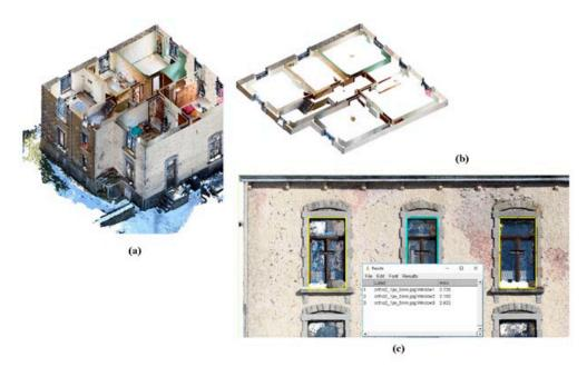
Figure 9. Building A surveyed with MVP: (a) model obtained by combining the interior and exterior reconstructions; (b) a cross-section through the whole-building 3D model; (c) drawings and measurements using an orthomosaic photo as support.
