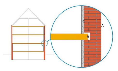
Figure 1. Parts of an exterior wall at risk of failure when installing internal insulation. (A) frost and discoloration of the façade surface, (B) rot in, and mould growth on, the beam ends, (C) mould and rot (if wood) on the interstitial materials surfaces and adjacent materials.
