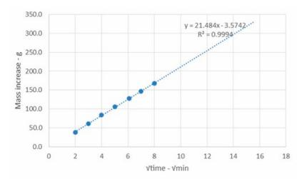
Figure 1. Typical sorptivity raw data for a carbonated NHL2 mortar cube.
