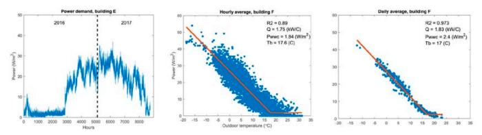
Figure 8. Building E, measured hourly values of power (left), results of hourly change-point model (middle) and daily change-point model (right).
