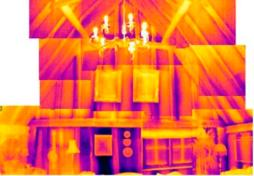
Figure 7. Interior thermography of north wall of drawing room. Source: Author's own, 2017.
