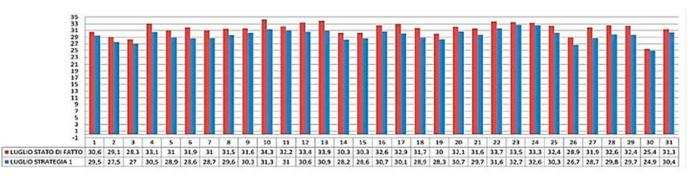
Figure 6. Explanatory diagram of the lowering of the monthly internal average temperature caused by the adoption of a shadowing strategy in July (blue column) compared to the actual situation (red column).
