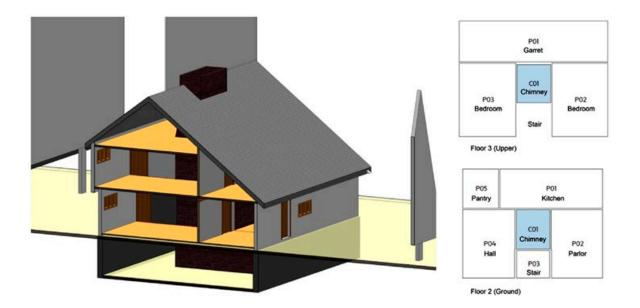
Figure 6. CAD: Revit Model of Ideal Saltbox House Figure 7. Second and Third Floor Room Delineation.
