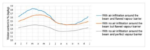
Figure 3. Impact of air infiltration around the beam end and of realistic flaws in airtightness for a configuration with cement lime plaster as external coating and cellulose wadding as insulation material. (Indicator A)
