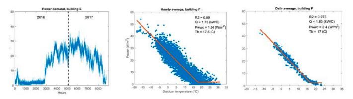
Figure 9. Building F, measured hourly values of power (left), results of hourly change-point model (middle) and daily change-point model (right).
