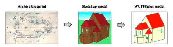
Figure 3. Scheme showing the creation of a building model in WUFI®plus starting from a blueprint.
