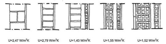
Figure 4. Façade solution and transmittance of the five Architectonic/Constructive Styles.
