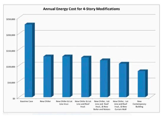
Figure 4. Effects of Upgrades to Building and Systems on Energy Costs for the Four-Story Building.
