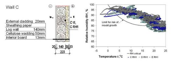
Figure 1. One section from six studied test walls (left) and temperature and RH conditions that are favourable for mould growth between log and insulation.
