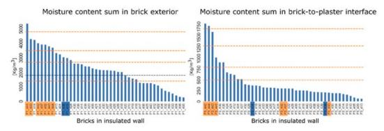
Figure 3. Ranking of bricks based on sum of moisture content at the exterior (left) and the brick-plaster surface (right) of an insulated  $1\frac{1}{2}$  brick thick SW oriented wall. Location Copenhagen, winter 2026–2027 (Dec 1 – Mar 1). Bricks marked with orange and blue boxes refer to the highest-ranking bricks in Figure 2.
