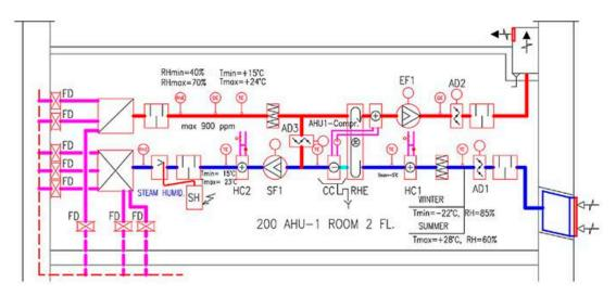
Figure 2. The principle of the Central AHU.
