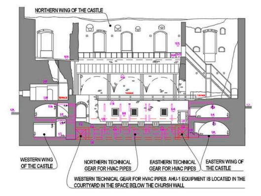
Figure 3. The first option for ventilation ducts.
