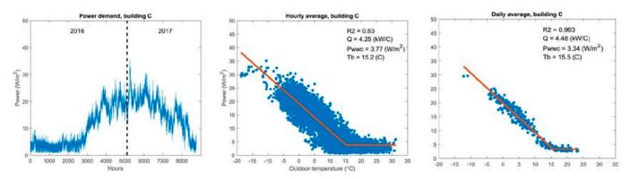
Figure 5. Building B, measured hourly values of power (left), results of hourly change-point model (middle) and daily change-point model (right).
