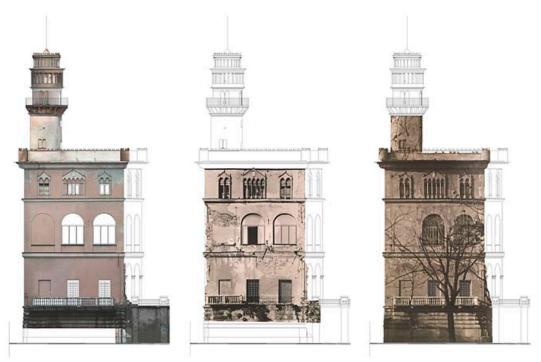
Figure 2. Different constructive phases, external plaster and openings: 2006, 1973, 1926.
