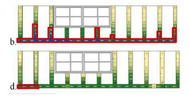
Figure 8. Surface moisture content (%) of timber-frame. Ground floor. Bedroom east wall (a.02/08/2016 and c.11/03/2017) Study north wall, (b.02/08/2016 and d.11/03/2017). Source: Author's own, 2017.
