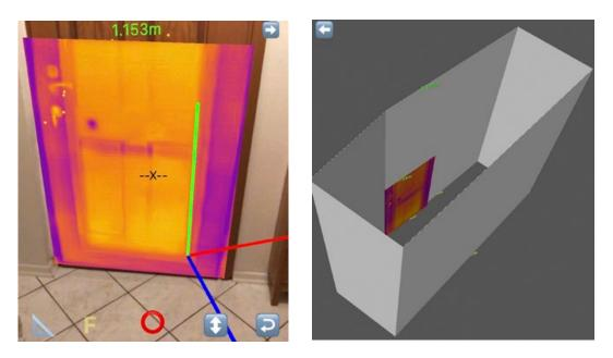
Figure 4. Overlapped images (left), 3D spatio-thermal model and calculated measurements (right).
