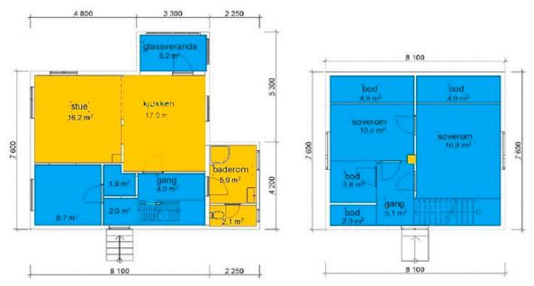
Figure 2. First and second floor in Villa Dammen. Yellow colour shows the area that is permanently heated, including the centred new brick stove. The wall between the two larger rooms in the first floor is removed. The basement is not shown and has not been included in the energy modelling. Second floor rooms are indirectly or intermittently heated.
