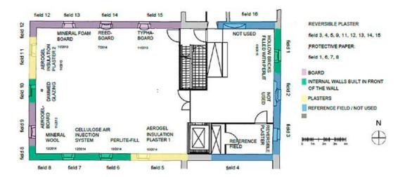
Figure 7. Interior insulation systems installed in the old cooperage with details of the insulation material and the installation time.
