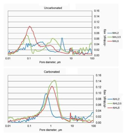
Figure 5. Pore size distributions of (upper) uncarbonated and (lower) carbonated mortars.
