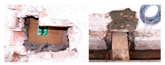
Figure 9. Variant N4/4b with fresh mortar in direct contact to the beam head (left) and. variant N5/3 with a lot of built in mortar (right). Photos: Fraunhofer Institute for Builing Physics IBP.
