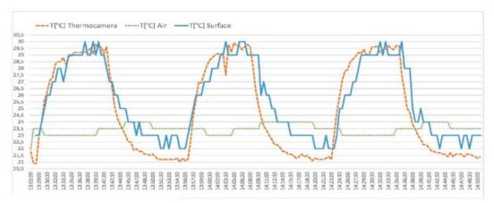
Figure 3. Graphic of the temperatures during three heating/cooling phases: the temperature of the tapestry surface, red line (by IRT), blue line (by contact probe); temperature of the side of the tapestry toward the wall and air trapped in the tapestry knots, green line (by data-logger).
