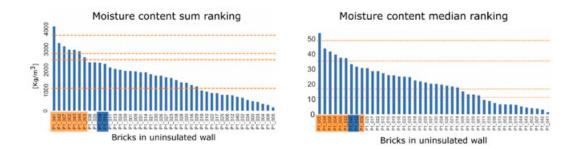
Figure 2. Ranking of bricks based on sum of moisture content (left) and moisture content median (right) at the exterior of a SW oriented 1½ brick thick wall without insulation. Location Copenhagen, winter 2026–2027 (Dec 1 to Mar 1). The seven highest-ranking brick types in the sum diagram (left), marked with orange, are in the median diagram (right) mixed with two other brick types marked with blue in both diagrams.
