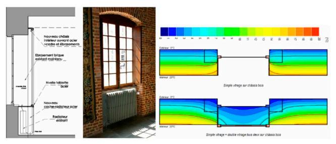
Figure 2. Installation of an over-frame and isotherms.
