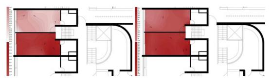
Figure 9. Temperature distribution before (left, 30.11.2015) and after (right, 22.2.2017) the pilot site.
