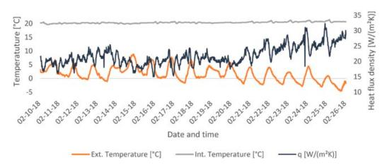
Figure 10. The hybrid WSN system makes it possible to monitor advanced variables remotely, such as the heat fluxes through walls.
