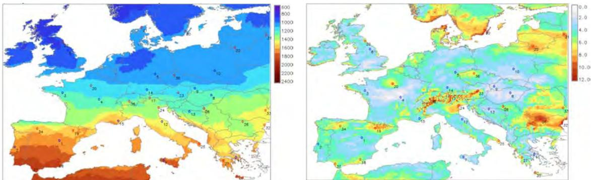
**Figure 2. Yearly sum of global irradiation on horizontal surface: (left) average of 6 databases: Meteonorm v.6, ESRA, PVGIS, NASA SSE v.6, Satel-Light and Helioclim-2 [kWh/m2]; (right) standard deviation of the values from 6 databases relative to the overall average [%].**
