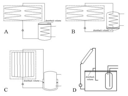
Fig. 2: Different implementations of the drainback concept.
