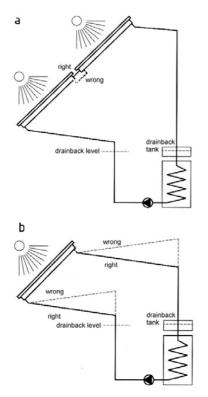
*Fig. 1: Examples of correctly, respectively wrongly designed drainback collector loops showing the basic principle of this technology and some of its constraints.*
