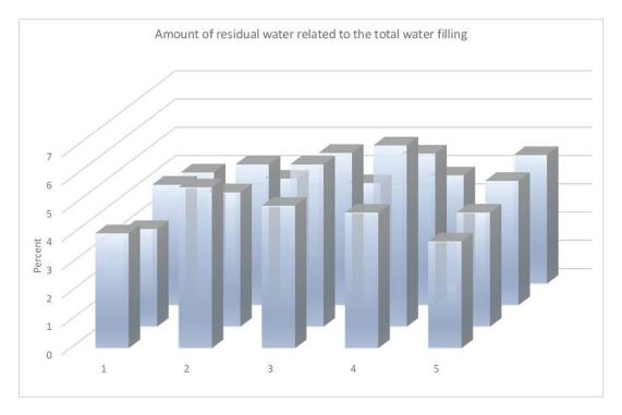
6.5 h freezing at -8 °C, min. 3.4 % residual water, max. 6.4 % residual water
