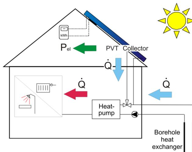
Fig. 1 Investigated system concept with the unglazed PVT collector integrated in a heat pump system with borehole heat exchanger
