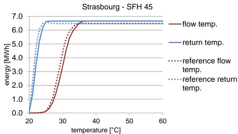
Figure 1. Temperature distribution of flow and return line of the radiator for the simulated system and the reference system in IEA Task 44 / Annex 38
