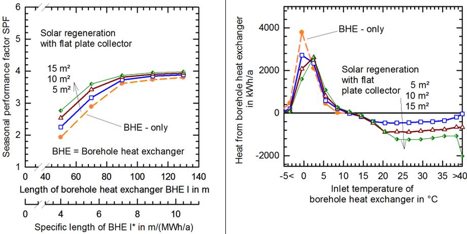
Figure 3. Impact of solar flat plate collector with 5, 10 and 15  $\text{m}^2$  on the seasonal performance factor SPF and the temperature distribution of the in system concept 1 the dashed line is without solar regeneration. The temperature distribution is given for a borehole heat exchanger length of 110 m.
