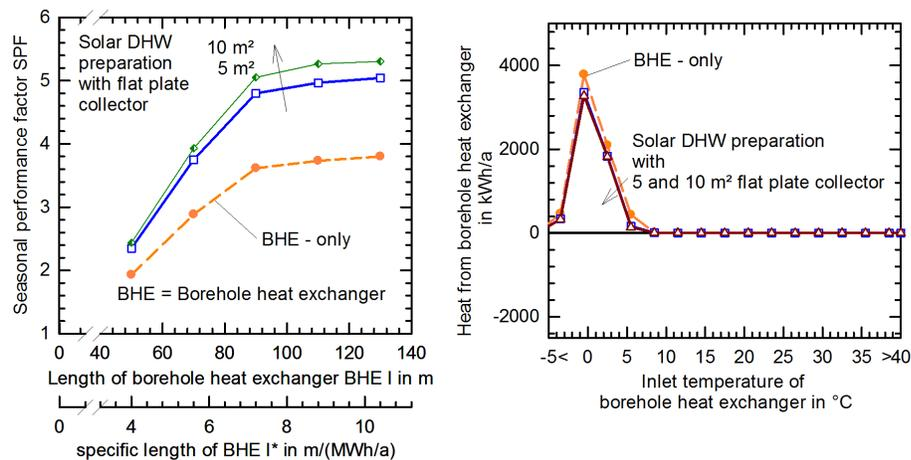
Figure 4. Impact of solar flat plate collector with 5 and 10 m<sup>2</sup> on the seasonal performance factor SPF (left) and the temperature distribution of the system concept 2 (right). The dashed line is without solar DHW preparation. The temperature distribution is given for a borehole heat exchanger length of 110 m.
