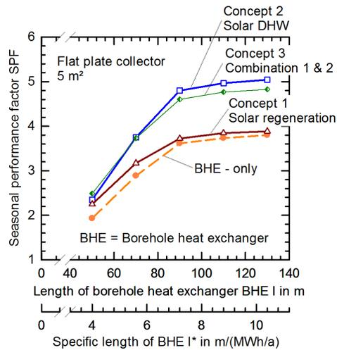
Figure 5. System performance of 5 m<sup>2</sup> flat plate collector for the system concepts one, two and three
