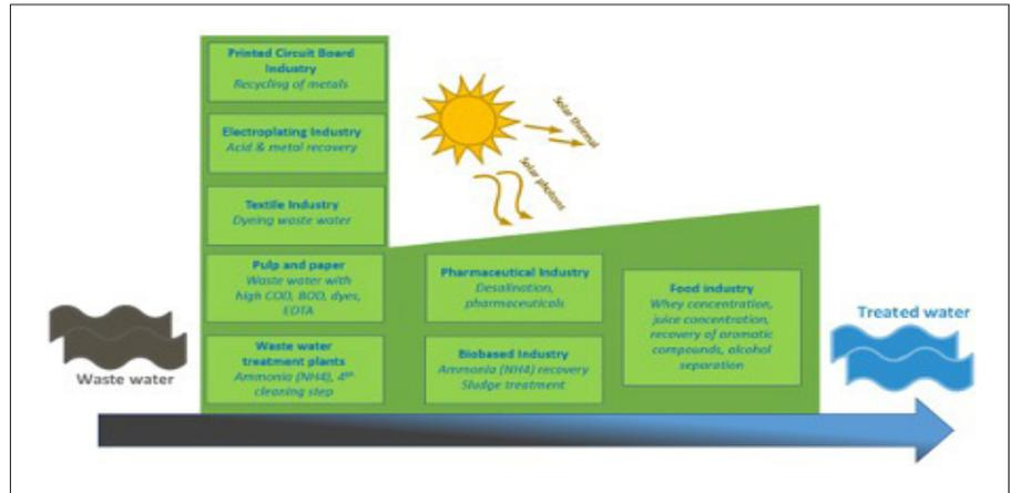
In terms of decontamination and disinfection systems, advanced oxidation processes (AOPs) for degrading contaminants in wastewater are available. Examples are photocatalysis or Photo-Fenton processes.
