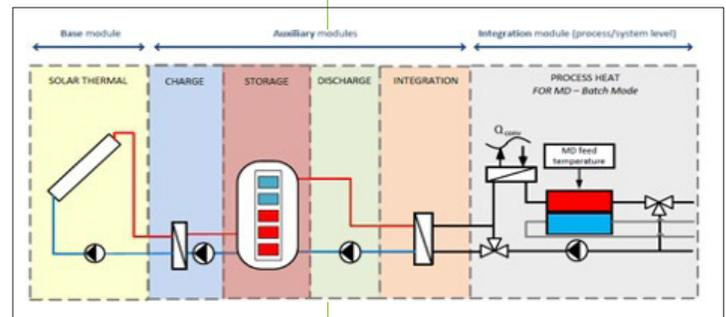
▲ Figure 4. Example of an integration concept combining solar thermal for the process heat supply of Membrane Distillation.
