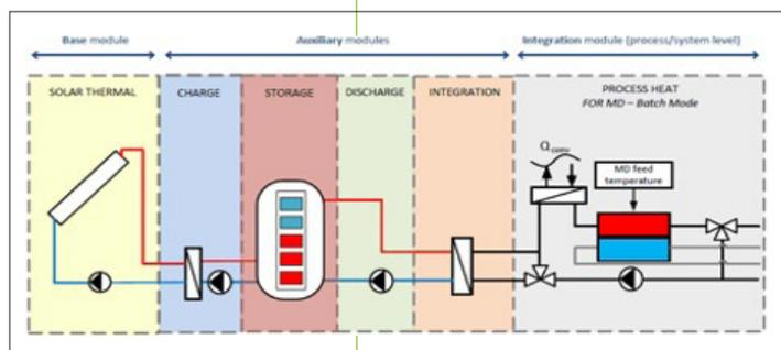
▲ Figure 4. Example of an integration concept combining solar thermal for the process heat supply of Membrane Distillation.
