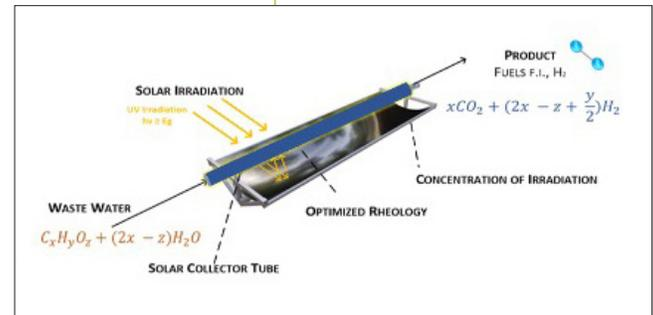
▲ Figure 3. Concept of the “Solar Reactor.” (Source: AEE INTEC)
