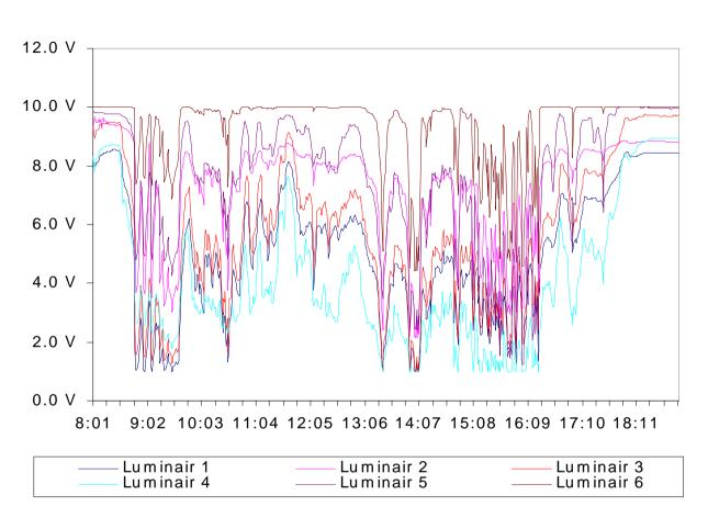
Figure 6 Voltage over regulator for six luminaires
