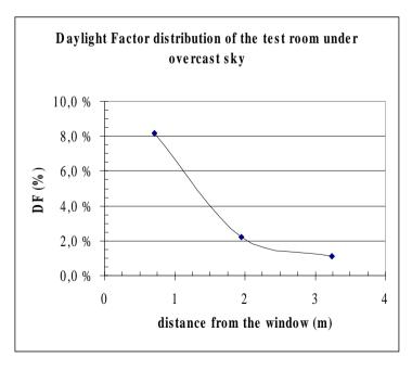
Fig.2. Measured daylight distribution in the test room
