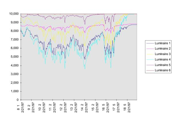
Figure 4 Voltage over regulator for six luminaires
