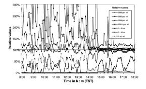
Figure 15 Relative values: power of luminaires, illuminances on working plane and facade illuminance, 15.05.99
