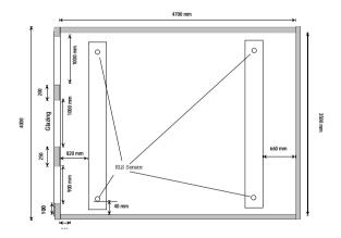
Figure 17 Luminaire and sensor position
