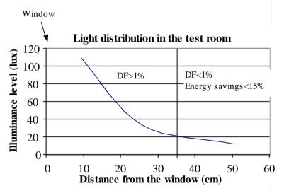
*Figure 2*: daylight distribution in the test room (the measurements and calculations have been done under overcast sky)
