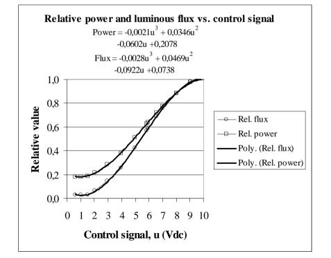
Fig. 3. Light output and power consumption of a 58W fluorescent lamp as a function of the control signal.
