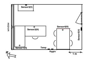
Figure 1: Layout of the room, including the position of the sensors
