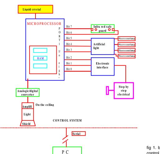
To change-To test control programs fig 1. block diagram of the control system
