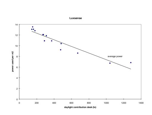
Figure 7, average used power per  $m^2$  as a function of the daylight contribution
