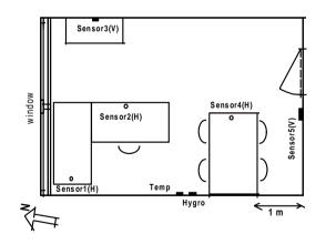
Figure 1: Layout of the room, including the position of the sensors.
