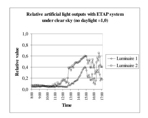
Fig. 4 Relative artificial need per luminaire with Etap ELS system. Reference levels (individual to each luminaire) are measured at night without daylight.
