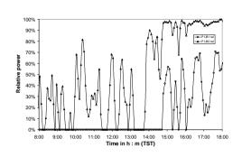
Figure 14 Relative power of luminaire rows, 15.05.99
