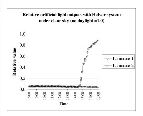
Fig. 5. Relative artificial need per luminaire with Helvar Mimo 2 system. Reference levels (individual to each luminaire) are measured at night without daylight. Table 1. Calculated average energy savings.
