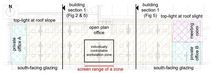
Figure 2. Floor plan of the Bartenbach R&D building.
