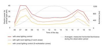
Figure 4. Comparison of the electric power for artificial light for different lighting zonings, supplemented by the averaged measured daylight-based illuminance values (data set from: 02.09. - 03.11.2020).
