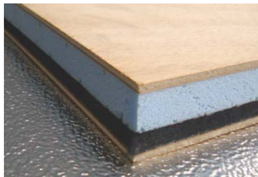
Figure 3.5-39 Composite panel with plywood, extruded polystyrene and aerogel fleece [115]
