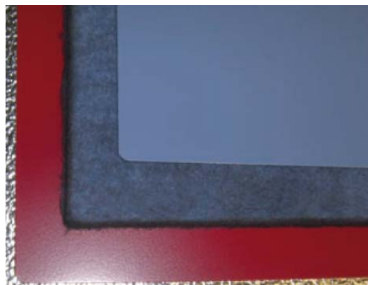
Figure 3.5-40 Composite panel with aerogel fleece and aluminium panels on either side [115]
