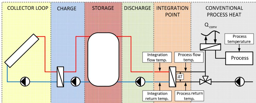
**Figure 9: General SHIP system for pre-heating with five subsections supplying an industrial heat consumer** (Helmke and Hess, in Muster-Slawitsch et al., 2015)
