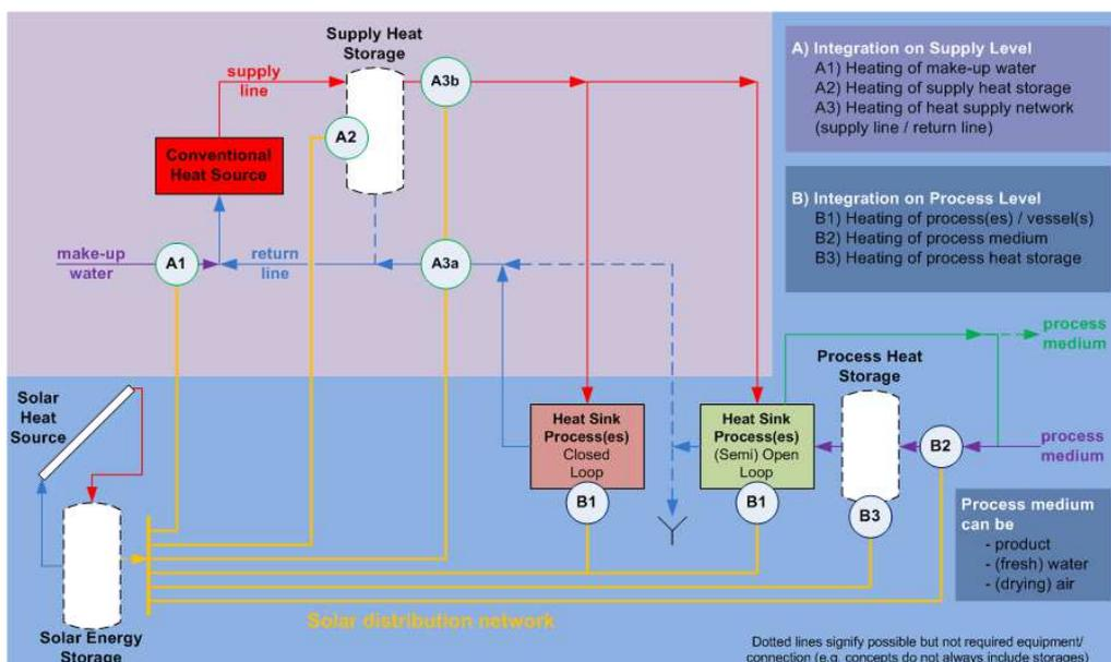
**Figure 1: Possible integration points for solar process heat** (MusterSlawitsch et al., 2015)
