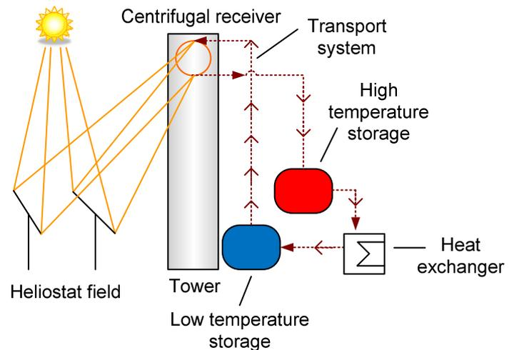
**Figure 15: Solar particle receiver – new high temperature concept** (Prosinecki, in Muster-Slawitsch et al., 2016)
