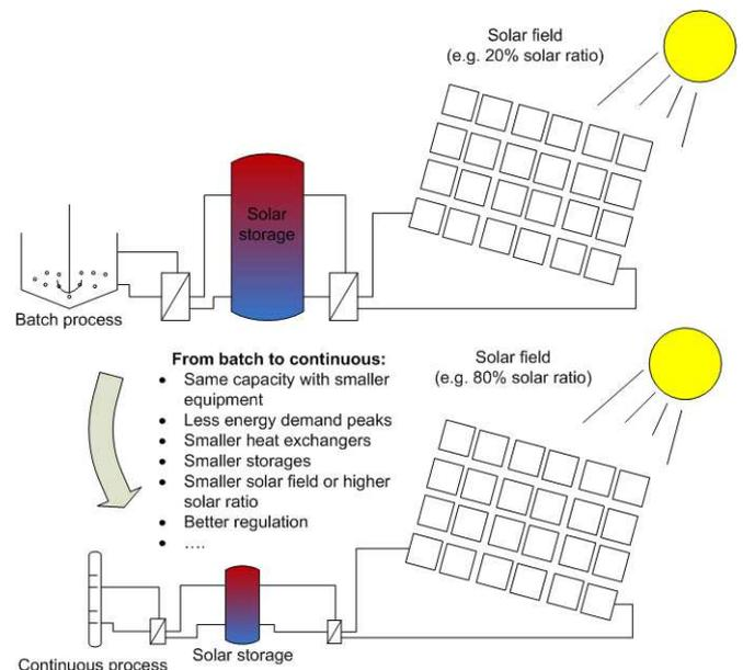
**Figure 16: effects on solar process heat by changing from batch to continuous processes (example for intensification strategies)**
