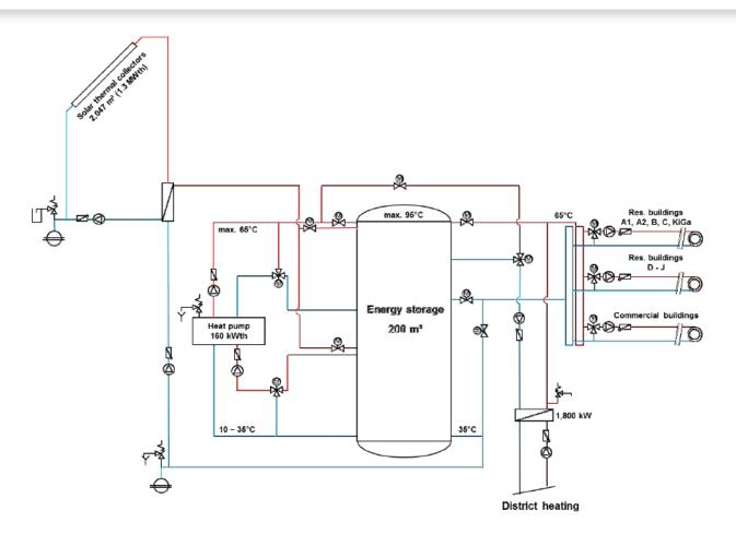
Figure 11. Hydraulic scheme of the heat supply system in Salzburg-Lehen (Source: AEE INTEC)
