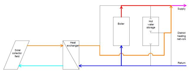
Figure 2. Indirect return-to-supply integration of ST
