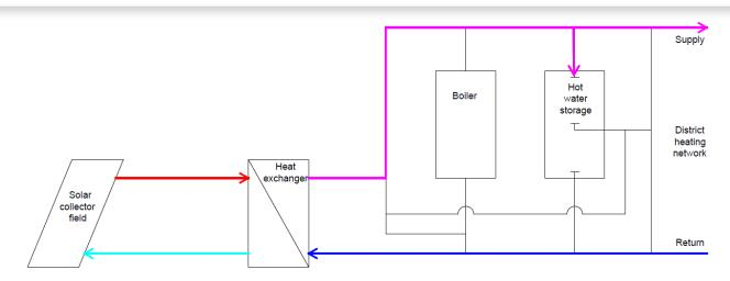
Figure 1. Return-to-supply integration of ST
