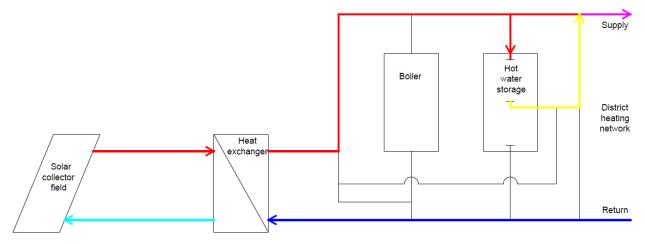
Figure 5. Integration of ST with storage as shunt
