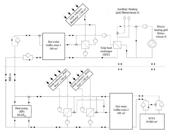
Figure 9. Hydraulic scheme of the SDH system in Crailsheim (Source: [3])
