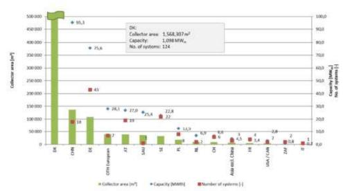
Large-scale systems for solar district heating—capacities and collector area installed and number of systems in 2020 (concentrating systems and PVT collectors add up to 162,784 m²). Source: Solar Heat Worldwide Report 2021
