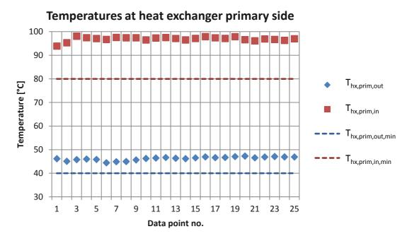
Fig.3.3.6. Temperature requirements fulfilled since  $T_{hx,prim,out}$  is above  $T_{hx,prim,out,min}$  (40 °C) and  $T_{hx,prim,in}$  is above  $T_{hx,prim,in,min}$  (80 °C) as required.
