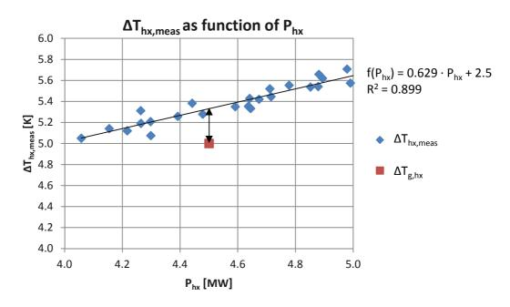
*Fig.3.3.5.* Temperature difference across heat exchanger as function of the transferred power. Guarantee point indicated with red square at 4.5 MW; 5 K. It is seen that in this case the guarantee is NOT fulfilled! Check of temperatures:
