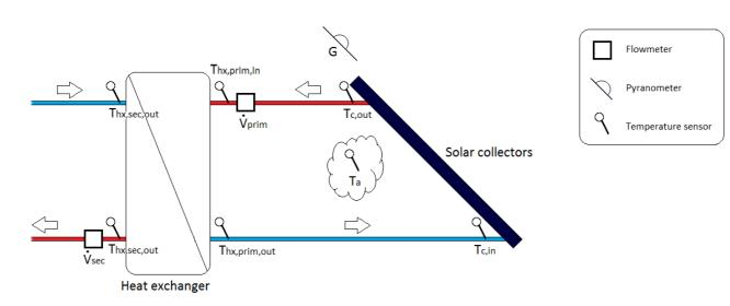
Fig. 3.3.2. Schematic drawing showing the measurement points.
