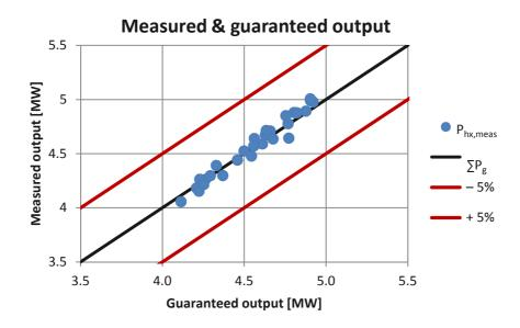
Fig. 3.3.4. Plot of measured thermal power point against corresponding guaranteed thermal power points.
