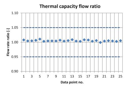
*Fig.3.3.7. Capacity flow rate ratio requirement fulfilled since the measurement points are between 0.95 and 1.05 as required.*
