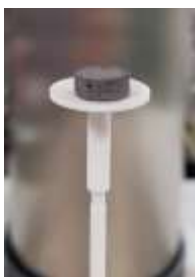
Figure 3. Cilindric porous pellets used for TG analysis.
