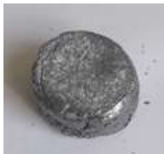
Figure 8. \text{SrCl}_2 impregnated into ENG.
