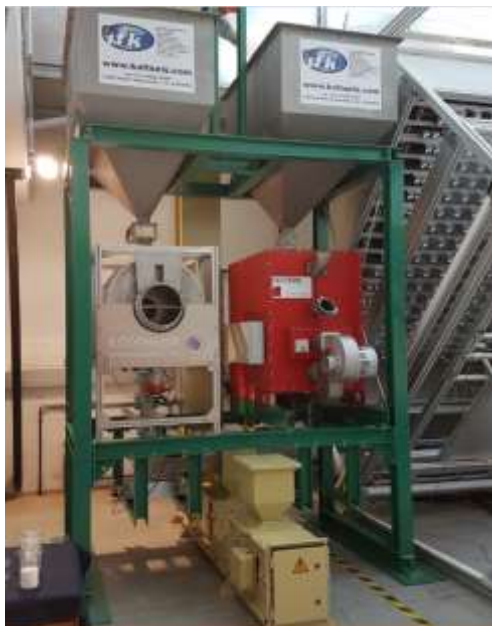
Figure 6 Rotating bed open heat storage prototype developed in Project OFFSOR.
