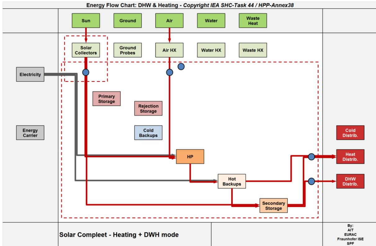
Figure 7: energy flow chart of S+HP system.
