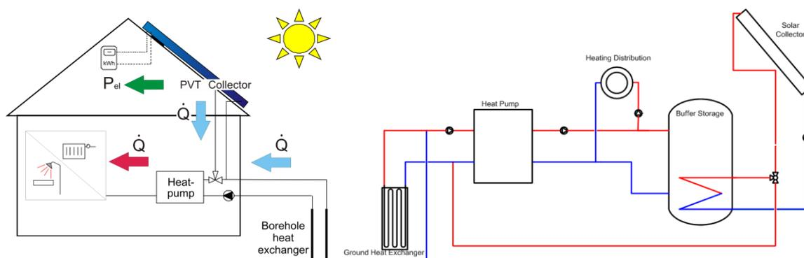
Figure 1: S+HP system: Example of a system including PV-T collectors and ground heat exchanger coupled with a water-to-water heat pump (source: ISFH and Fraunhofer ISE).
