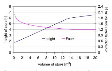
Figure 5.2: height of store and UA correction factor Fcorr<sub>UAstore,A</sub> as a function of the store volume.
