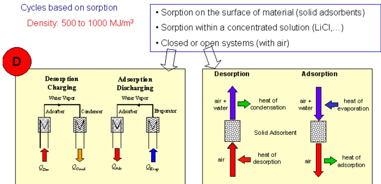
Figure 10 – Germany: Principle of a sorption storage in closed (left) or open (right) systems during charging and discharging phase
