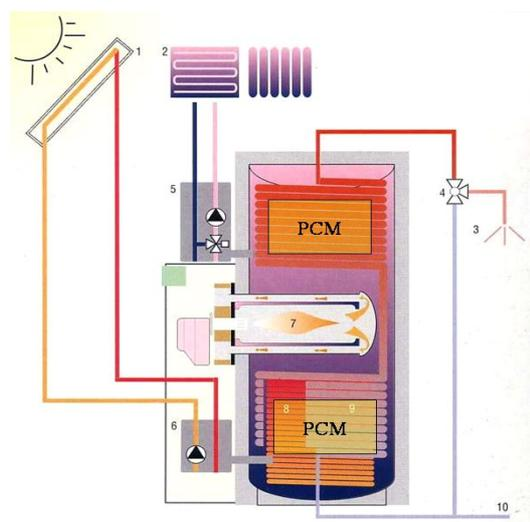
Figure 7 – Switzerland: Where to place a PCM storage in a water tank to improve the storage performance ? Theroretical and experimental studies are carried out
