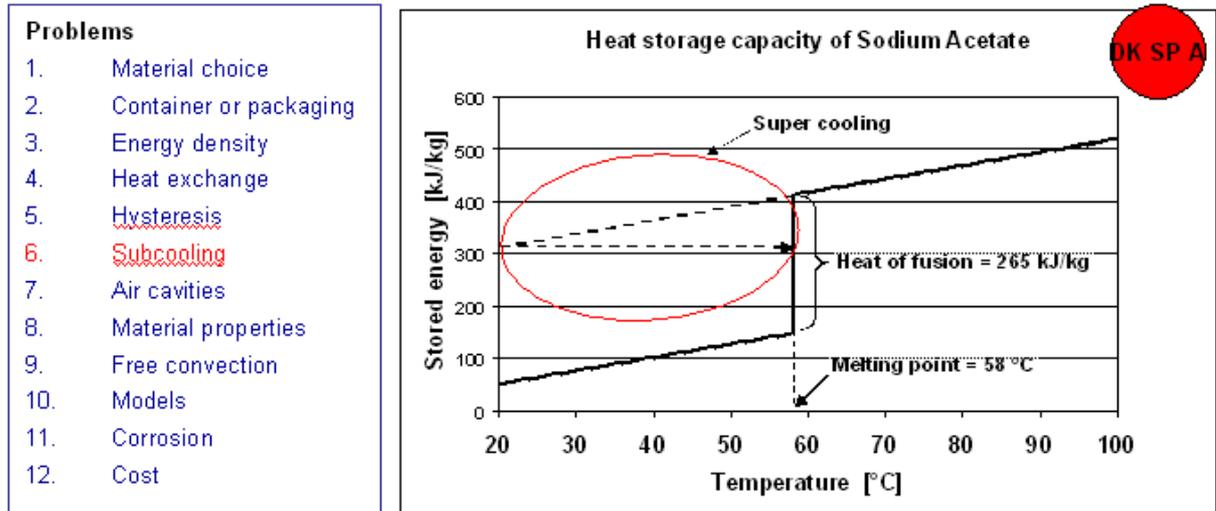
Figure 8 – Main issues of PCM storage and the subcooling effect that must be modelled to accurately predict the performance of a PCM storage
