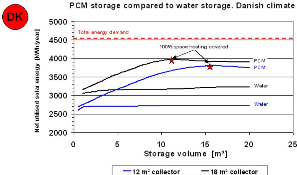
Figure 9 – Denmark: The subcooling effect might be an advantage for seasonal storage according to preliminary simulations
