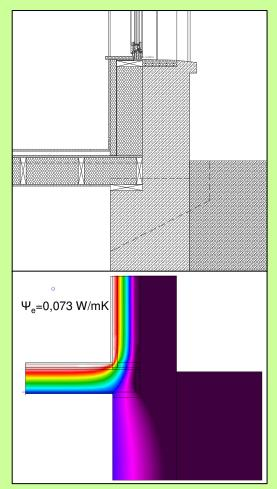
Construction detail and thermal conductivity image of the connection floor slab - façade
