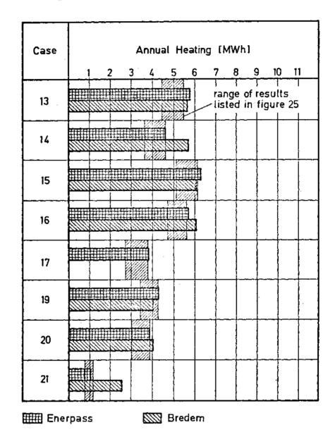
Fig. 44 Annual heating loads of Phase II calculated by design tools with weather conditions of DENVER. Hatched areas indicate the ranges of results obtained by detailed building energy analysis simulation models (BLAST, DOE 2.1C, SERIRES, HTB 2, ESP) in Fig. 25.
