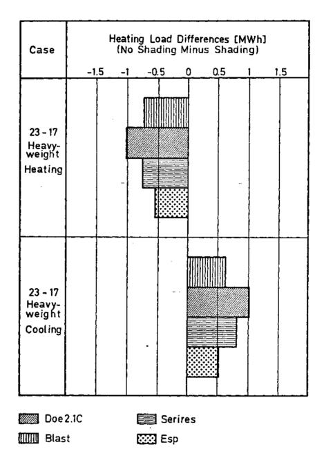
Fig. 34 Differences in annual heating loads of Phase II between no shading and shading calculated by detailed building energy analysis simulation models with weather conditions of DENVER.
