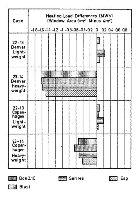
Fig. 35 Differences in annual heating loads of Phase II between 9 m' and 4 m' south window area calculated by detailed building energy analysis simulation models with weather conditions of DENVER and COPENHAGEN.
