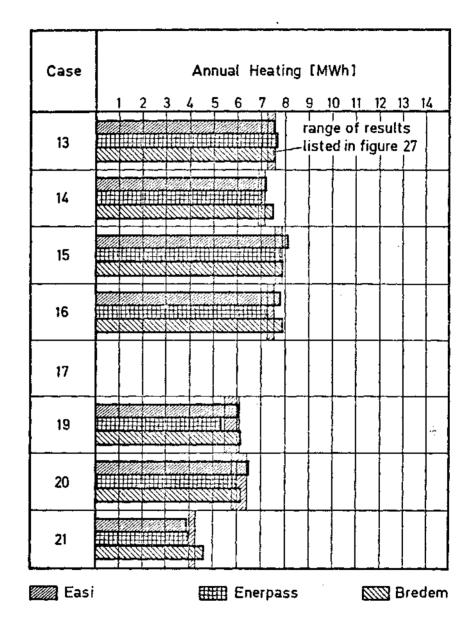
Fig. 42 Annual heating loads of Phase II calculated by design tools with weather conditions of COPENHAGEN. Hatched areas indicate the ranges of results obtained by detailed building energy analysis simulation models (BLAST, DOE 2.1C, SERIRES, HTB 2, ESP) in Fig. 27.
