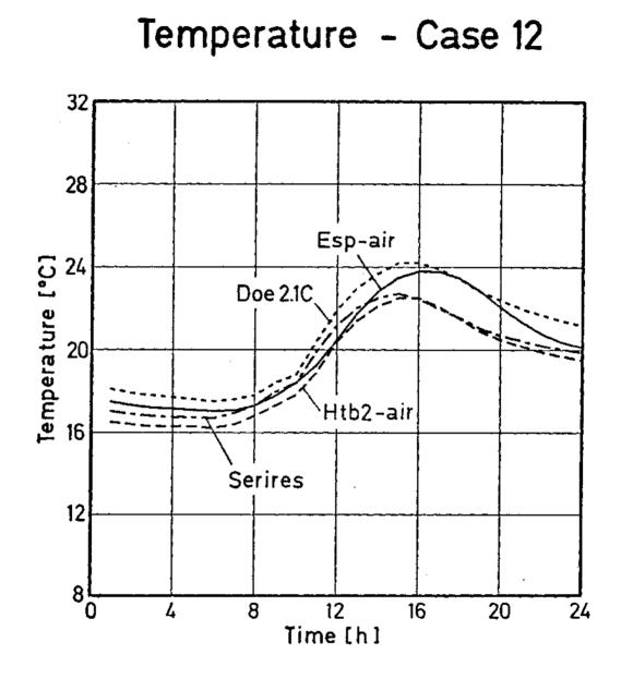
Fig. 16 Hourly free-floating temperatures of Case 12 (heavyweight building) calculated by detailed building energy analysis simulation models with weather conditions of COPENHAGEN, May 30.
