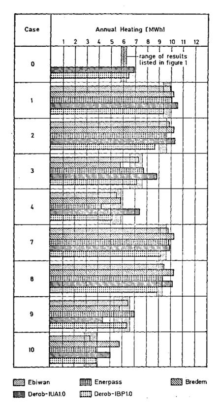
Fig. 17 Annual heating loads of Phase I calculated by design tools with weather conditions of DENVER. Hatched areas indicate the ranges of results obtained by detailed building energy analysis simulation models (BLAST, DOE 2.1C, SERIRES, HTB 2, ESP) in Fig. 1.
