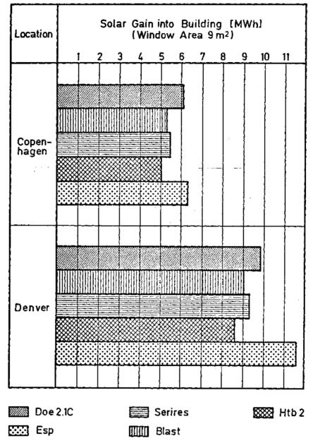
Fig. 8 Annual solar input of cases with window area 9 m' calculated by detailed building energy analysis simulation models with weather conditions of COPENHAGEN and DENVER.
