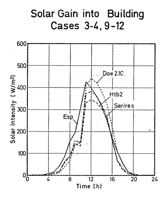
Fig. 12 Hourly solar gain into building of Cases 3-4 and 9-12 calculated by detailed building energy analysis simulation models with weather conditions of COPENHAGEN, May 30.
