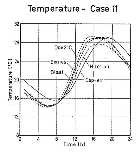
Fig. 13 Hourly free-floating temperatures of Case 11 (lightweight building) calculated by detailed building energy analysis simulation models with weather conditions of DENVER, May 30.
