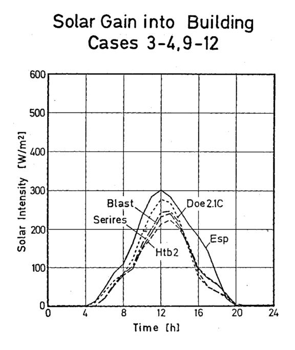
fig. 11 Hourly solar gain into building of Cases 3-4 and 9-12 calculated by detailed building energy analysis simulation models with weather conditions of DENVER, May 30.
