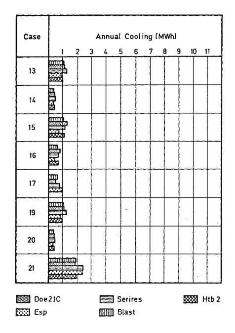
Fig. 26 Annual cooling loads of Phase II calculated by detailed building energy analysis simulation models with weather conditions of DENVER.
