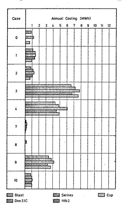
Fig. 2 Annual cooling loads of Phase I calculated by detailed building energy analysis simulation models with weather conditions of DENVER.
