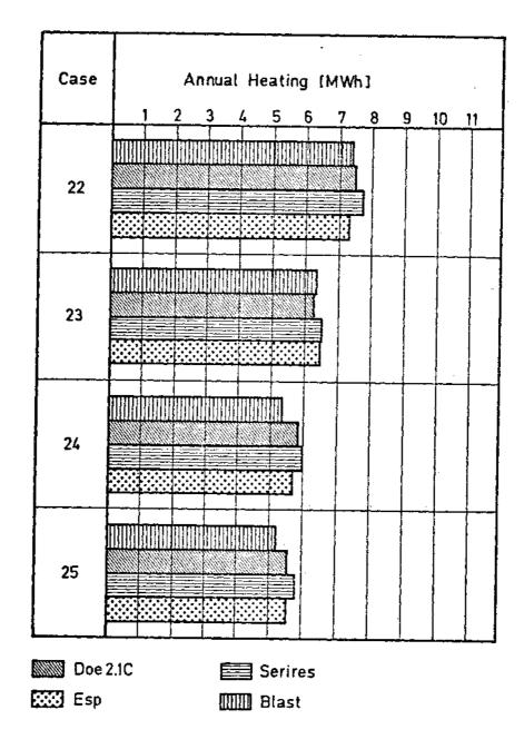
Fig. 31 Annual heating loads of Phase II calculated by detailed building energy analysis simulation models with weather conditions of COPENHAGEN.
