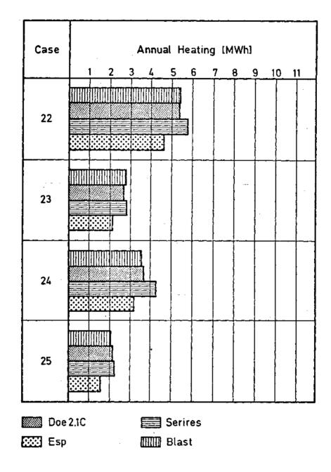
Fig. 29 Annual heating loads of Phase II calculated by detailed building energy analysis simulation models with weather conditions of DENVER.
