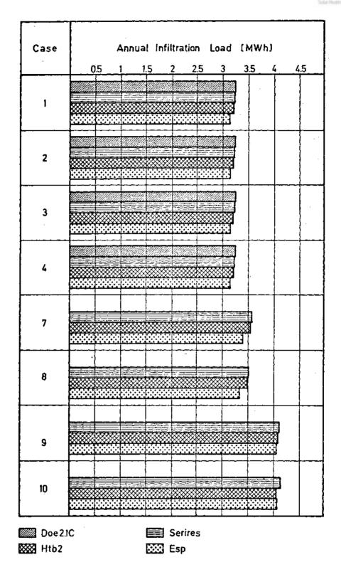
Fig. 6 Annual infiltration loads of Phase I calculated by detailed building energy analysis simulation models with weather conditions of DENVER.
