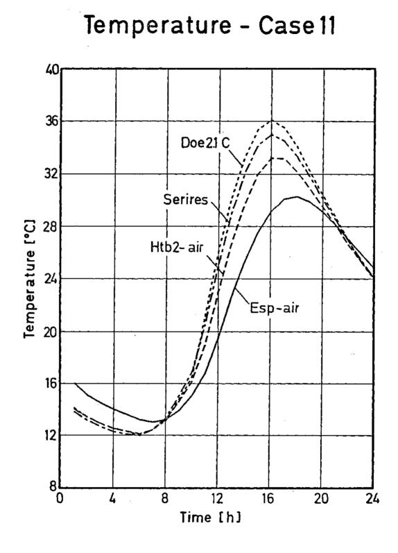
Fig. 14 Hourly free-floating temperatures of Case 11 (lightweight building) calculated by detailed building energy analysis simulation models with weather conditions of COPENHAGEN, May 30.
