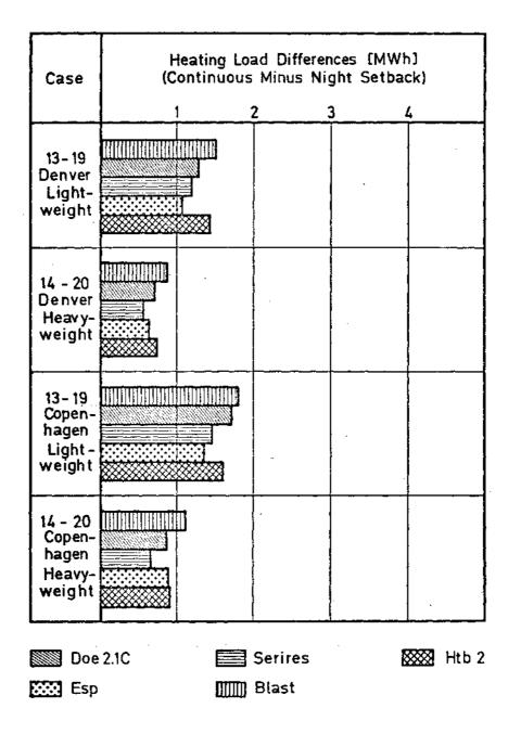
Fig. 33 Differences in annual heating loads of Phase II between continuous and night setback heating modes calculated by detailed building energy analysis simulation models with weather conditions of DENVER and COPENHAGEN.
