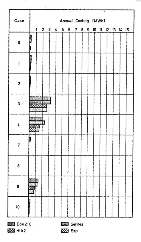
Fig. 4 Annual cooling loads of Phase I calculated by detailed building energy analysis simulation models with weather conditions of COPENHAGEN.
