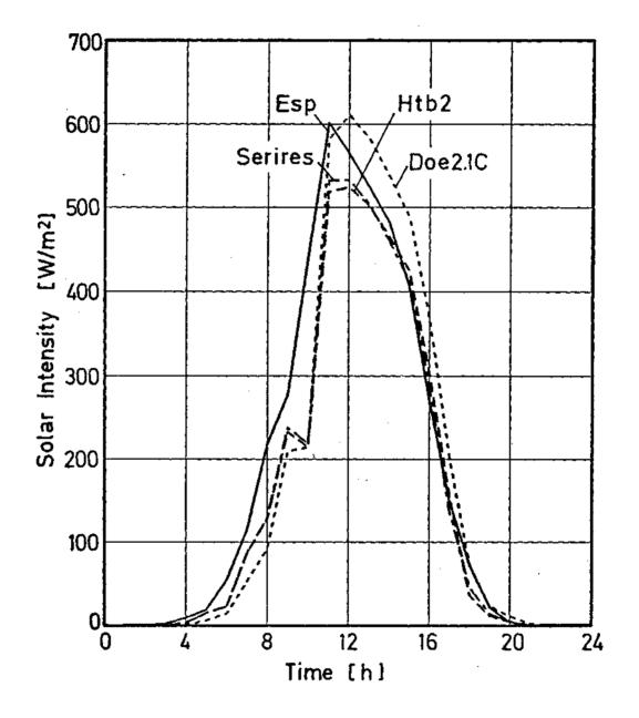
Fig. 10 Hourly solar radiation incident on the external south facing surface calculated by detailed building energy analysis simulation models with weather conditions of COPENHAGEN, May 30.
