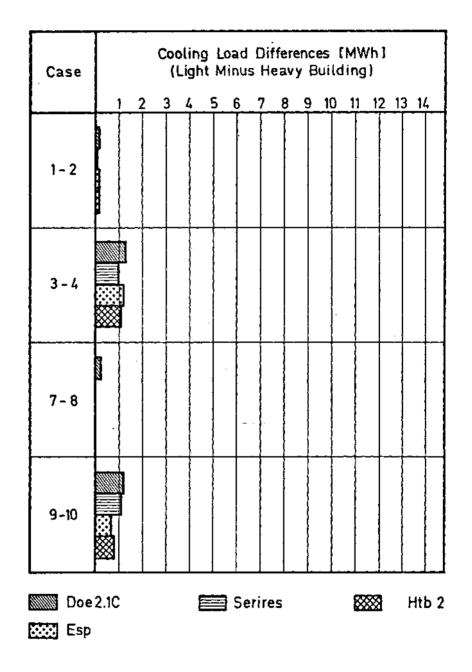
Fig. 24 Differences in annual cooling loads of Phase I between light and heavyweight buildings calculated by detailed building energy analysis simulation models with weather conditions of COPENHAGEN.
