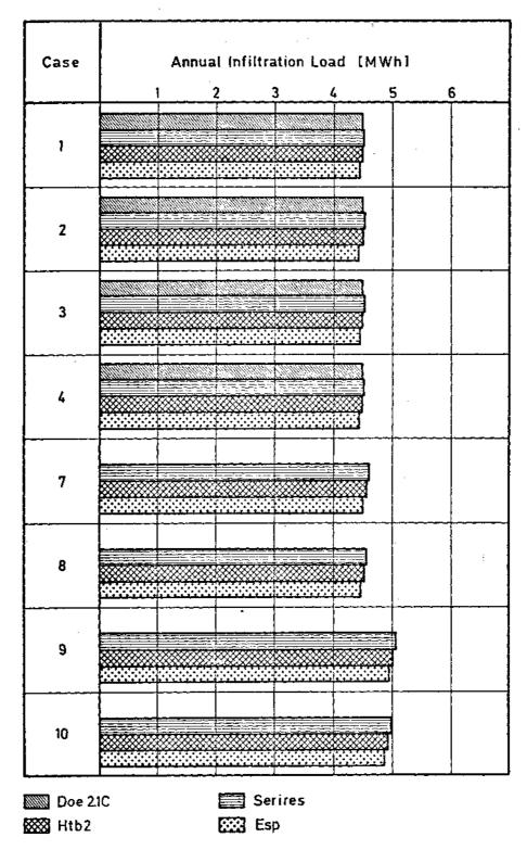
Fig. 7 Annual infiltration loads of Phase I calculated by detailed building energy analysis simulation models with weather conditions of COPENHAGEN.
