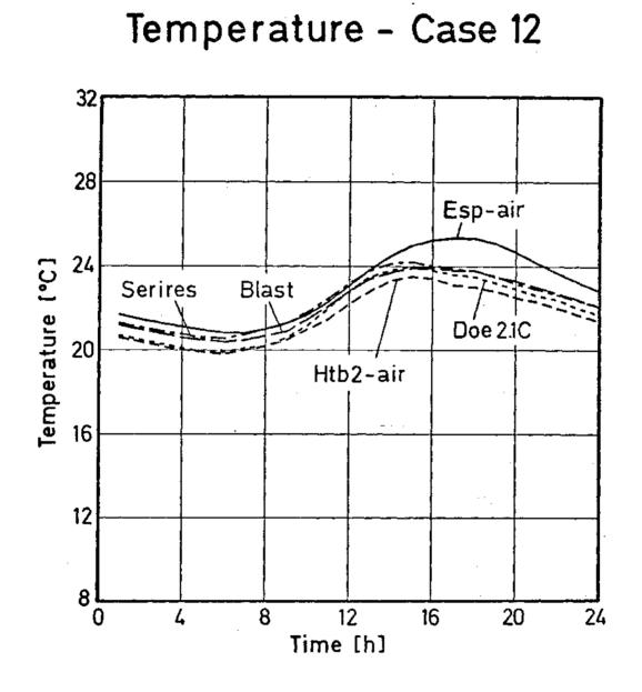
Fig. 15 Hourly free-floating temperatures of Case 12 (heavyweight building) calculated by detailed building energy analysis simulation models with weather conditions of DENVER, May 30.
