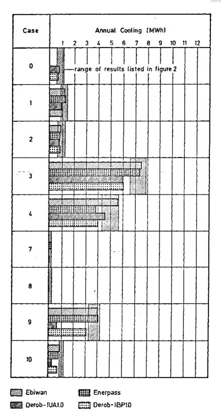
Fig. 18 Annual cooling loads of Phase I calculated by design tools with weather conditions of DENVER. Hatched areas indicate the ranges of results obtained by detailed building energy analysis simulation models (BLAST, DOE 2:1C, SERIRES, HTB 2, ESP) in Fig. 2.
