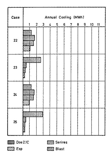
Fig. 32 Annual cooling loads of Phase II calculated by detailed building energy analysis simulation models with weather conditions of COPENHAGEN.
