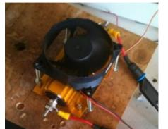
PV power (500 W) feeds an asynchron triple phase Motor which drives a generator
